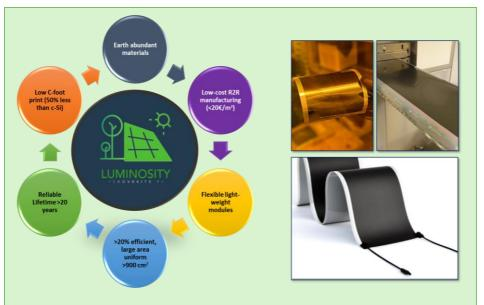
Figure 1 Principal advantages of LUMINOSITY technology and the prototype R2R coated layers on flexible FTO foil (top-right) to produce the envisioned product (bottom-right).
