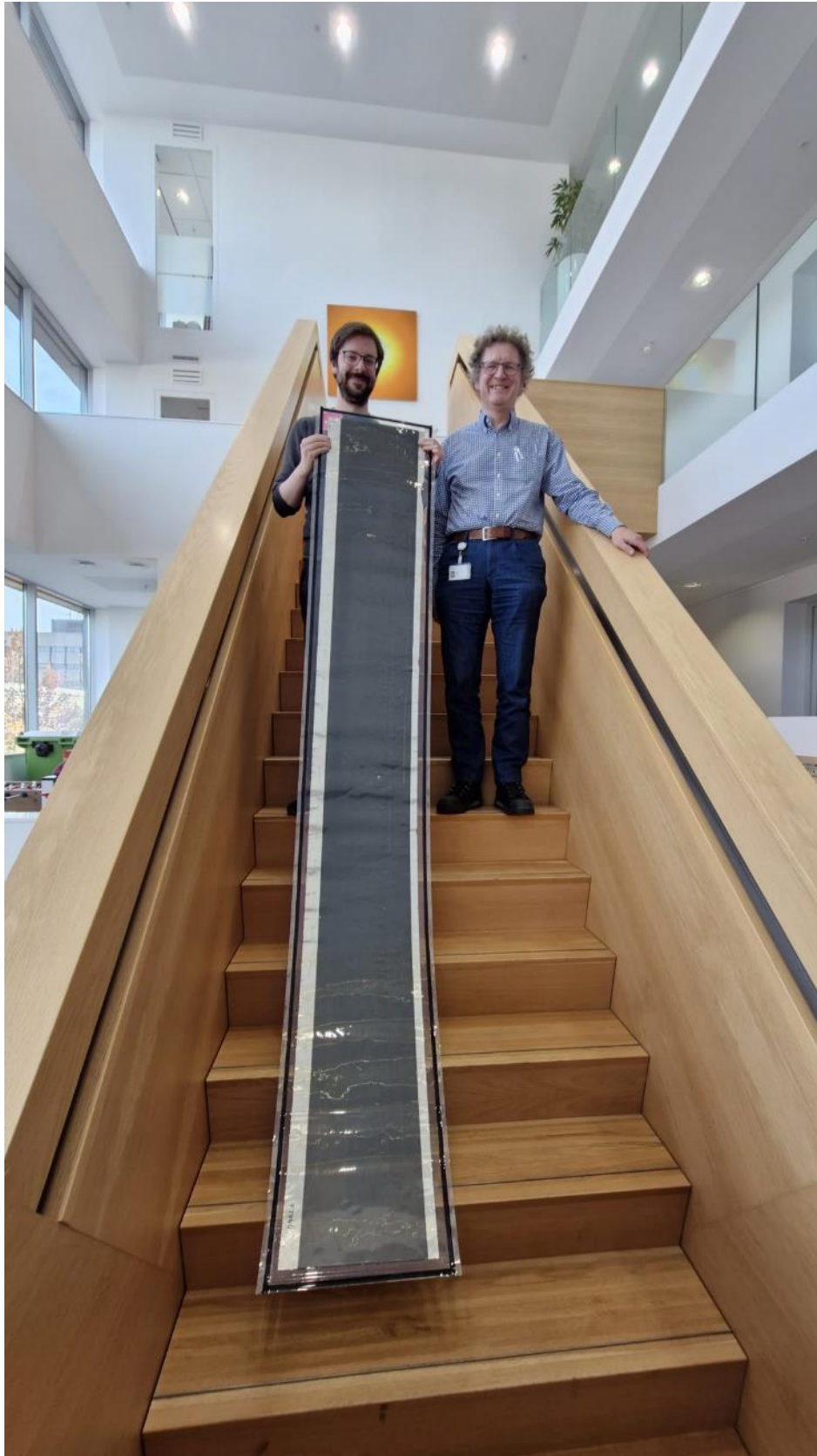
Figure 6 Demonstrator of an encapsulated perovskite semi-fabricate foil, produced by R2R techniques (R2R APCVD at HyET, R2R SD at TNO, R2R encapsulation at TNO). The total length of the coated foil is 2.5 meters, the coating area is 7500 cm 2 , the total length of the encapsulated demonstrator is 3 meters.
