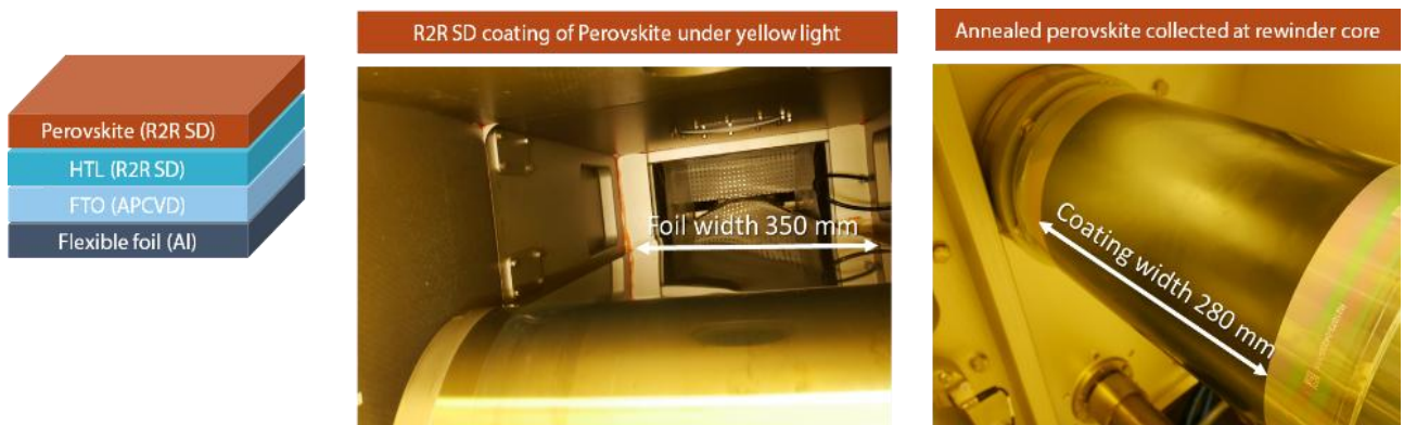
Figure 3 Ambient coating of Perovskite via R2R-SD technique. Coating is done under yellow light conditions in the clean room environment.
