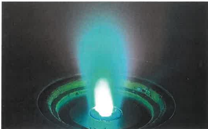
Evaporation of cesium iodide using an anodic arc. Image: Fraunhofer FEP
