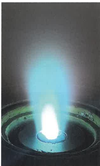
Evaporation of cesium iodide using an anodic arc
